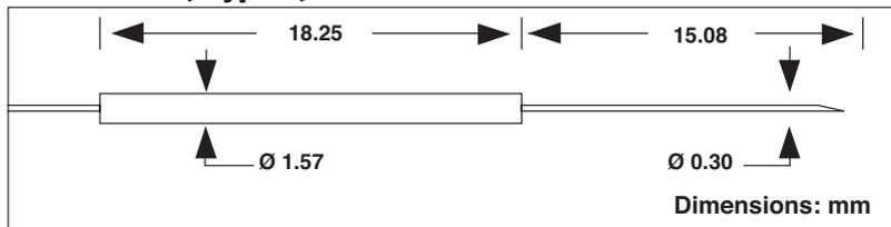
**Model HYP2, Type T, Ø 0.81mm Needle**
