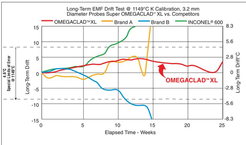
Super OMEGA CLAD® XL Probes are an excellent choice for high temperature measurement. They provide very low drift at high temperatures as compared to conventional Inconel and Stainless Steel sheathed probes. They are available in both K and N thermocouple calibrations. Omega offers probes in a variety of styles.
