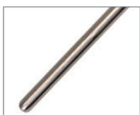
A thermocouple probe consists of thermocouple wire housed inside a metal or ceramic tube. The wall of the tube is referred to as the sheath of the probe. Common sheath materials include stainless steel and
