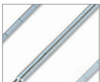
A beaded wire thermocouple is the simplest form of thermocouple. It consists of two pieces of thermocouple wire joined together with a welded bead. Because the bead of the thermocouple is exposed,
