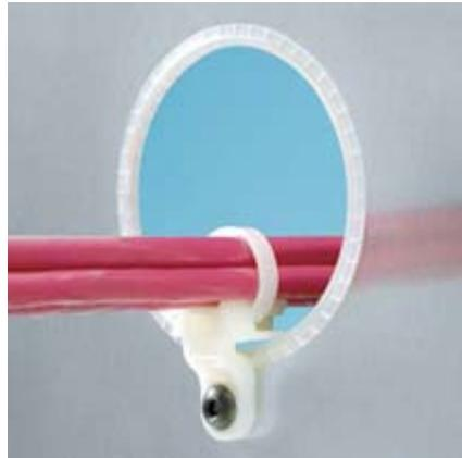
Used to secure wire bundles which run through bulkhead lightening holes .87" (22.1mm) diameter or larger, and keeps the bundles away from sharp edges. Only one screw rivet or self-tapping screw needed.
