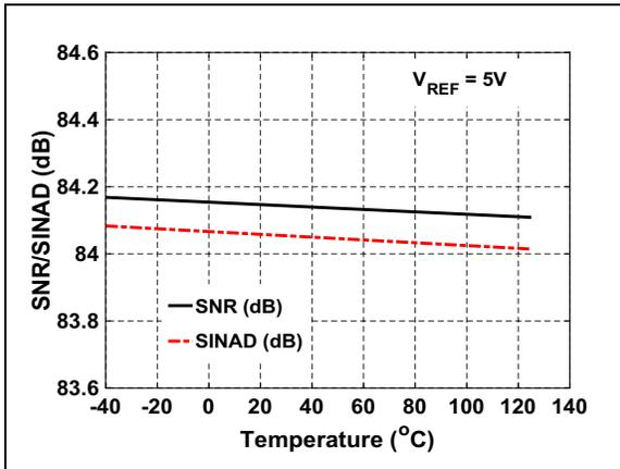
FIGURE 3-14: SNR/SINAD vs. Temperature:  $V_{REF} = 5\text{V}$ .
