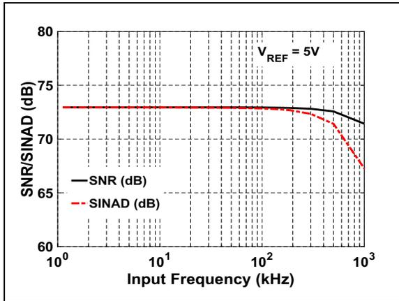
**FIGURE 4-19:** SNR/SINAD vs. Input Frequency:  $V_{IN} = -1\text{ dBFS}$
