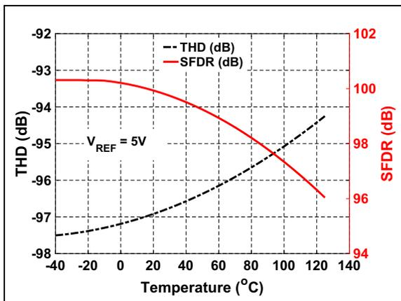
**FIGURE 4-20:** THD/SFDR vs. Temperature:  $V_{REF} = 5\text{V}$ .
