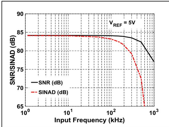
**FIGURE 3-19:** SNR/SINAD vs. Input Frequency:  $V_{IN} = -1\text{ dBFS}$ .
