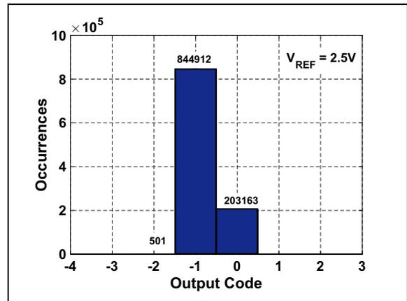
**FIGURE 3-29:** Shorted Input Histogram:  $V_{REF} = 2.5\text{V}$ .
