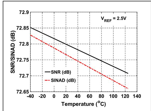
**FIGURE 4-17:** SNR/SINAD vs. Temperature:  $V_{REF} = 2.5\text{V}$ .
