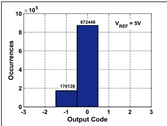
**FIGURE 4-26:** Shorted Input Histogram:  $V_{REF} = 5\text{V}$ .
