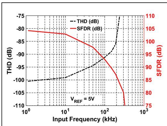
**FIGURE 2-21:** THD/SFDR vs. Input Frequency:  $V_{REF} = 5\text{V}$ .
