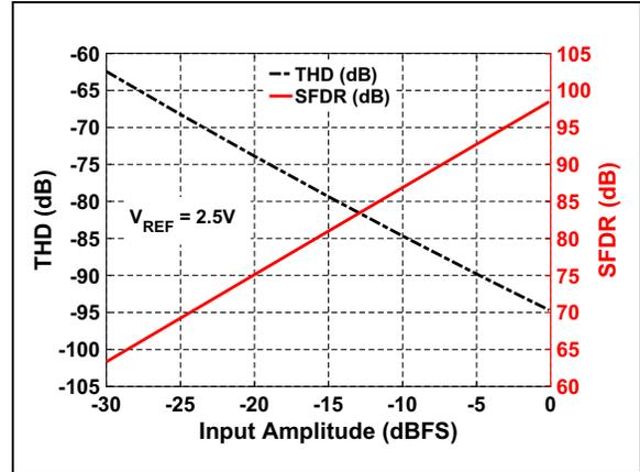
**FIGURE 4-28:** THD/SFDR vs. Input Amplitude:  $V_{REF} = 2.5\text{V}$ .
