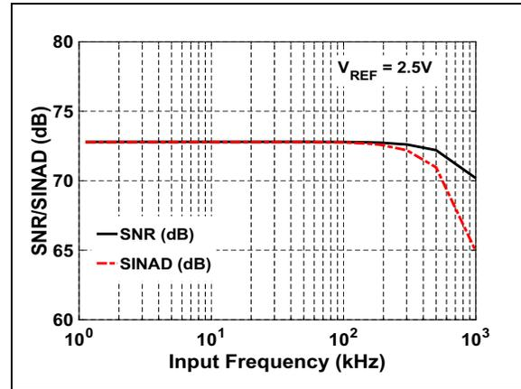
**FIGURE 4-22:** SNR/SINAD vs. Input Frequency:  $V_{IN} = -1\text{ dBFS}$ .
