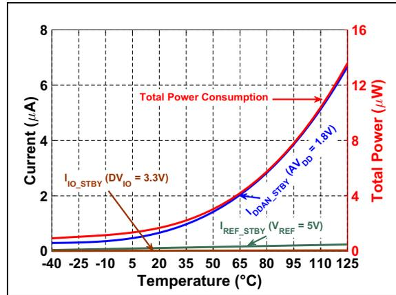
**FIGURE 3-34:** Power Consumption vs. Temperature during Shutdown.
