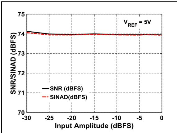
**FIGURE 4-15:** SNR/SINAD vs. Input Amplitude:  $f_{IN} = 10\text{ kHz}$ .
