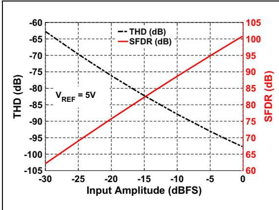
**FIGURE 4-25:** THD/SFDR vs. Input Amplitude:  $V_{REF} = 5\text{V}$ .
