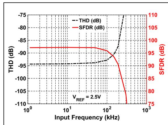
**FIGURE 4-24:** THD/SFDR vs. Input Frequency:  $V_{REF} = 2.5\text{V}$ .
