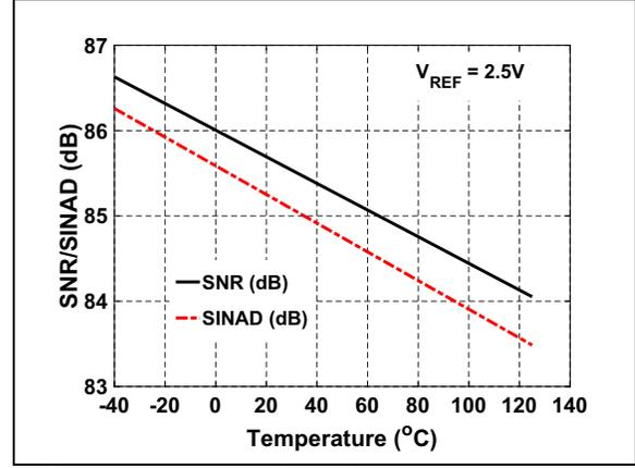
FIGURE 2-17: SNR/SINAD vs. Temperature:  $V_{REF} = 2.5\text{V}$ .
