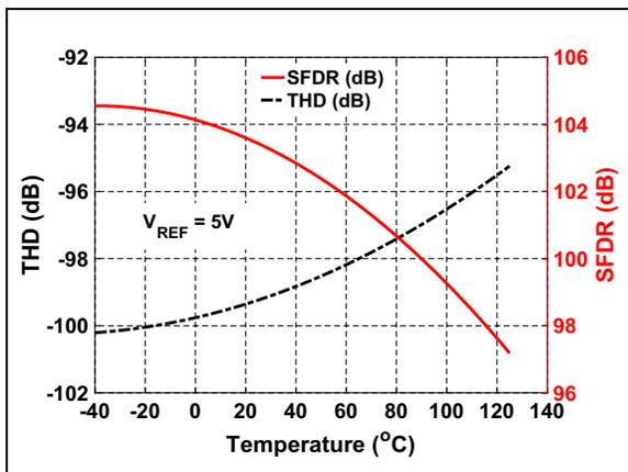
**FIGURE 3-20:** THD/SFDR vs. Temperature:  $V_{REF} = 5\text{V}$ .
