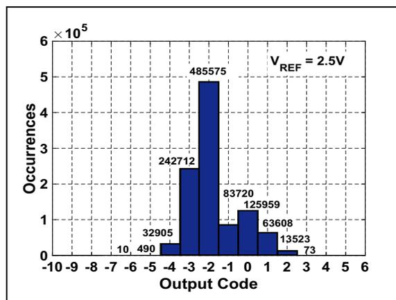
**FIGURE 2-29:** Shorted Input Histogram:  $V_{REF} = 2.5\text{V}$ .
