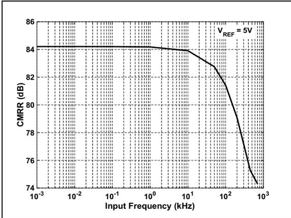
**FIGURE 2-31:** CMRR vs. Input Frequency:  $V_{REF} = 5\text{V}$ .
