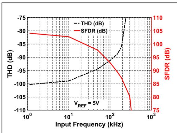
**FIGURE 3-21:** THD/SFDR vs. Input Frequency:  $V_{REF} = 5\text{V}$ .
