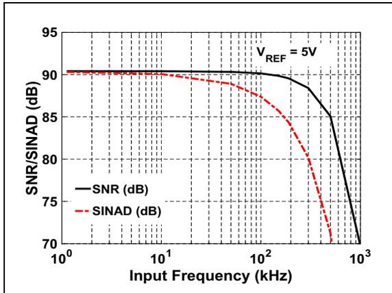
**FIGURE 2-19:** SNR/SINAD vs. Input Frequency:  $V_{IN} = -1\text{ dBFS}$ .
