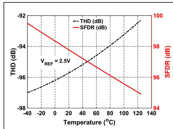
**FIGURE 3-23:** THD/SFDR vs. Temperature:  $V_{REF} = 2.5\text{V}$ .
