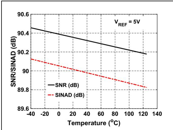
FIGURE 2-14: SNR/SINAD vs. Temperature:  $V_{REF} = 5\text{V}$ .
