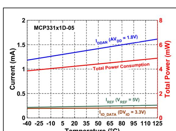
**FIGURE 2-36:** Power Consumption vs. Temperature:  $C_{LOAD\_SDO} = 20\text{ pF}$ .
