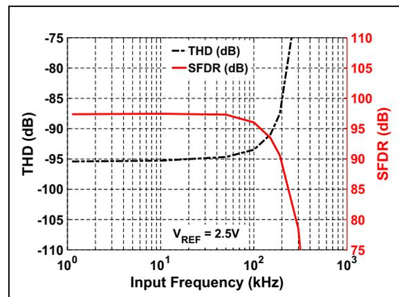
**FIGURE 2-24:** THD/SFDR vs. Input Frequency:  $V_{REF} = 2.5\text{V}$ .
