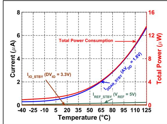
**FIGURE 4-34:** Power Consumption vs. Temperature during Shutdown.
