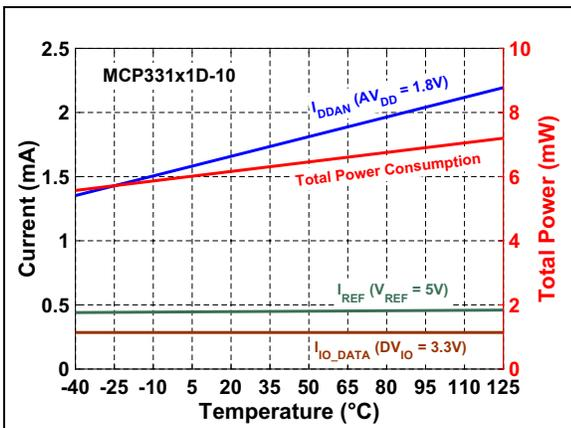
**FIGURE 3-33:** Power Consumption vs. Temperature:  $C_{LOAD\_SDO} = 20\text{ pF}$ .
