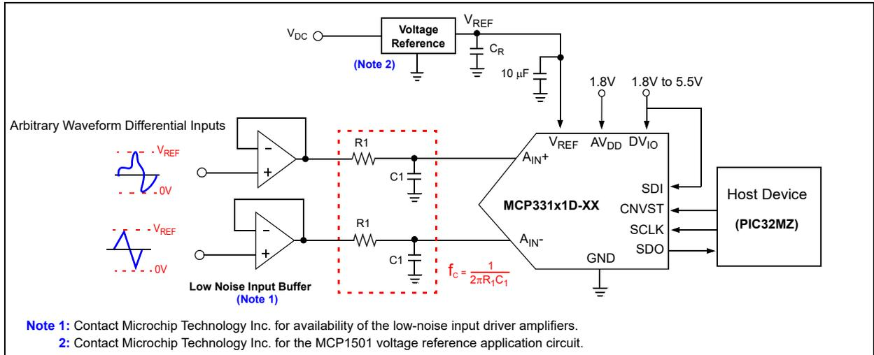
**FIGURE 6-4:** Input Configuration for Arbitrary Waveform Input Signals.
