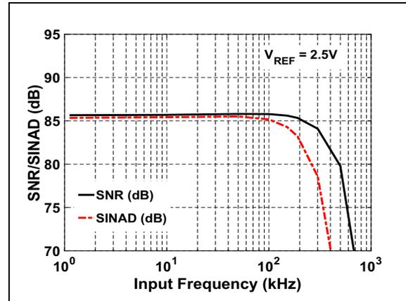
**FIGURE 2-22:** SNR/SINAD vs. Input Frequency:  $V_{IN} = -1\text{ dBFS}$ .
