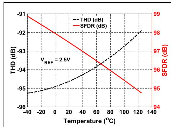
**FIGURE 4-23:** THD/SFDR vs. Temperature:  $V_{REF} = 2.5\text{V}$ .
