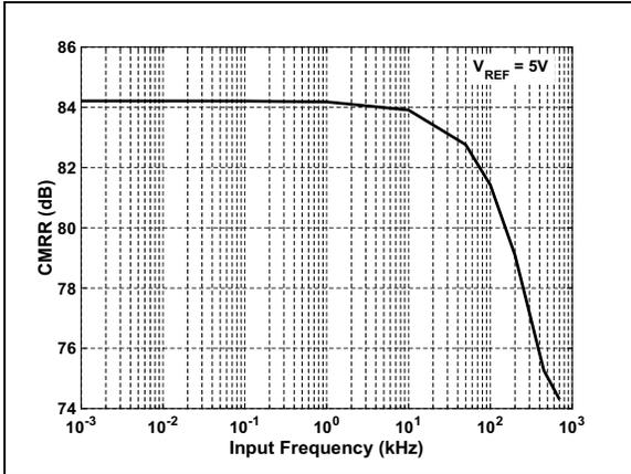
**FIGURE 4-31:** CMRR vs. Input Frequency:  $V_{REF} = 5\text{V}$ .
