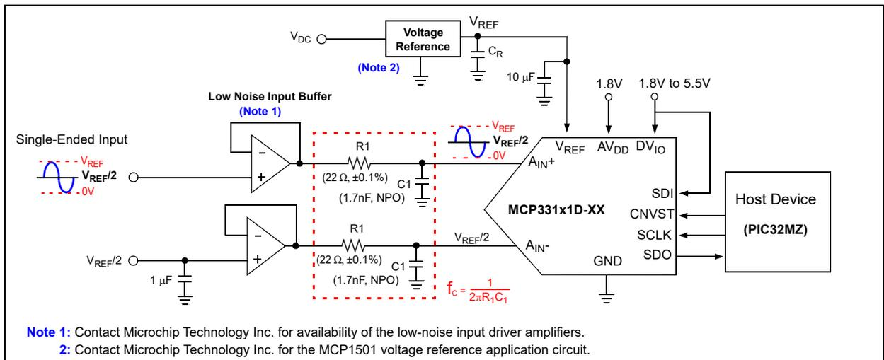
**FIGURE 6-5:** Pseudo-Differential Bipolar-Input Configuration for Single-Ended Input Signal.
