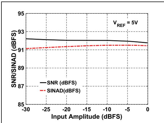
FIGURE 2-15: SNR/SINAD vs. Input Amplitude:  $f_{IN} = 10\text{ kHz}$ .
