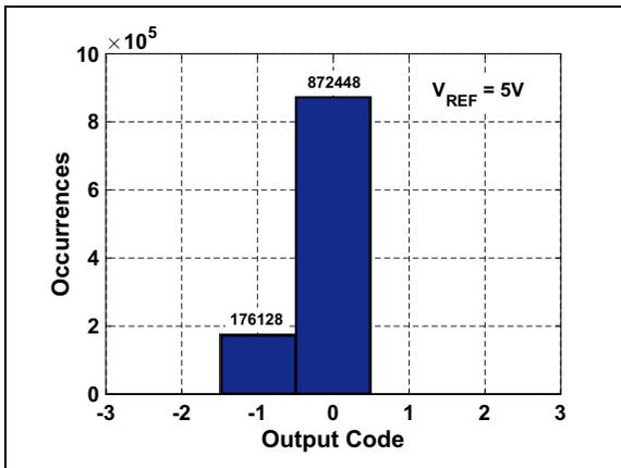
**FIGURE 3-26:** Shorted Input Histogram:  $V_{REF} = 5\text{V}$ .
