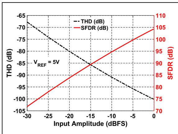
**FIGURE 2-25:** THD/SFDR vs. Input Amplitude:  $V_{REF} = 5\text{V}$ .
