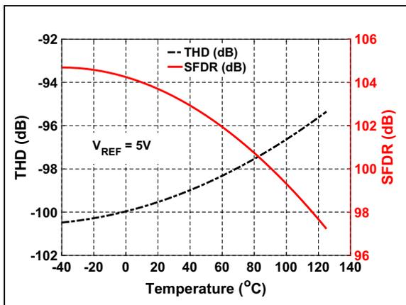
**FIGURE 2-20:** THD/SFDR vs. Temperature:  $V_{REF} = 5\text{V}$ .
