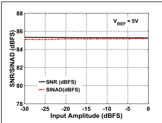
FIGURE 3-15: SNR/SINAD vs. Input Amplitude:  $f_{IN} = 10\text{ kHz}$ .
