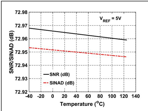
**FIGURE 4-14:** SNR/SINAD vs. Temperature:  $V_{REF} = 5\text{V}$ .
