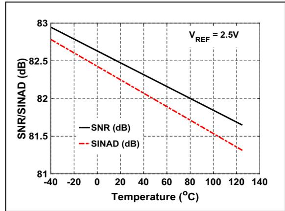
FIGURE 3-17: SNR/SINAD vs. Temperature:  $V_{REF} = 2.5\text{V}$ .
