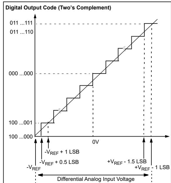
**FIGURE 6-11: Ideal Transfer Function for Fully-Differential Input Signal.**
