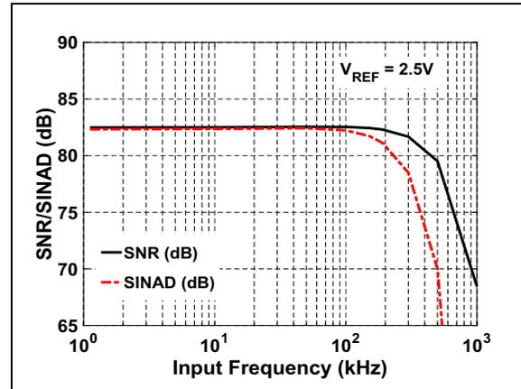
**FIGURE 3-22:** SNR/SINAD vs. Input Frequency:  $V_{IN} = -1\text{ dBFS}$ .
