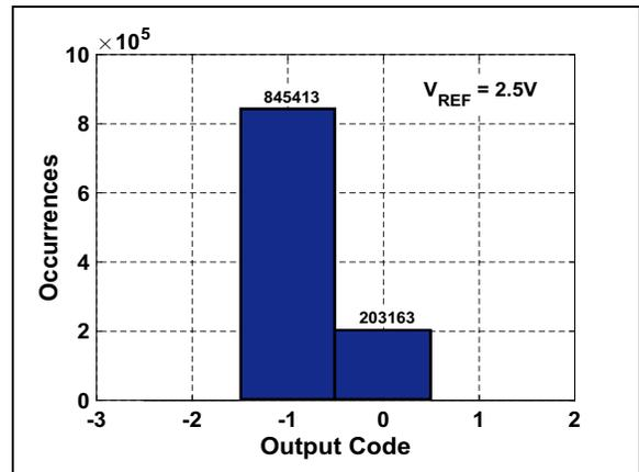
**FIGURE 4-29:** Shorted Input Histogram:  $V_{REF} = 2.5\text{V}$ .
