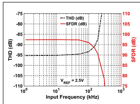
**FIGURE 3-24:** THD/SFDR vs. Input Frequency:  $V_{REF} = 2.5\text{V}$ .
