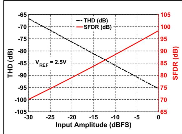
**FIGURE 3-28:** THD/SFDR vs. Input Amplitude:  $V_{REF} = 2.5\text{V}$ .
