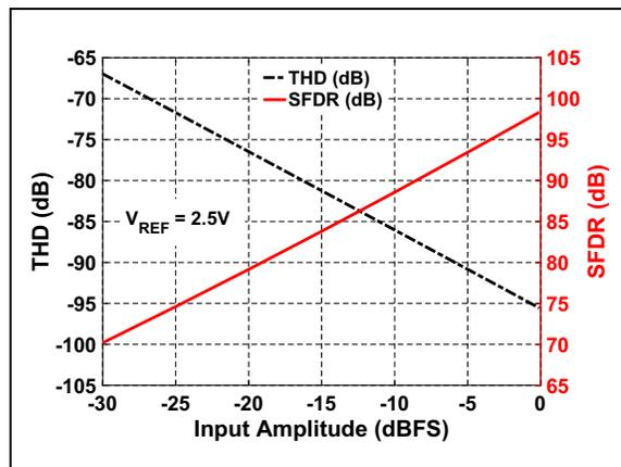
**FIGURE 2-28:** THD/SFDR vs. Input Amplitude:  $V_{REF} = 2.5\text{V}$ .
