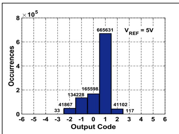
**FIGURE 2-26:** Shorted Input Histogram:  $V_{REF} = 5\text{V}$ .
