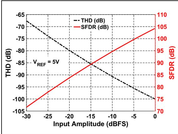
**FIGURE 3-25:** THD/SFDR vs. Input Amplitude:  $V_{REF} = 5\text{V}$ .
