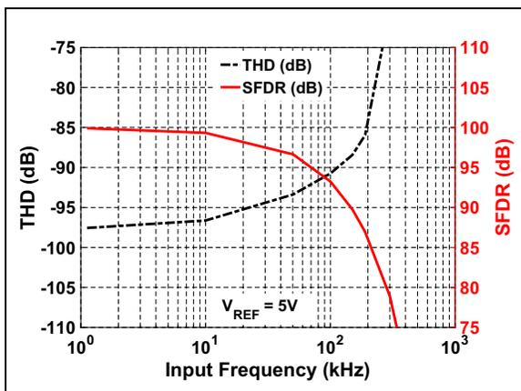
**FIGURE 4-21:** THD/SFDR vs. Input Frequency:  $V_{REF} = 5\text{V}$ .
