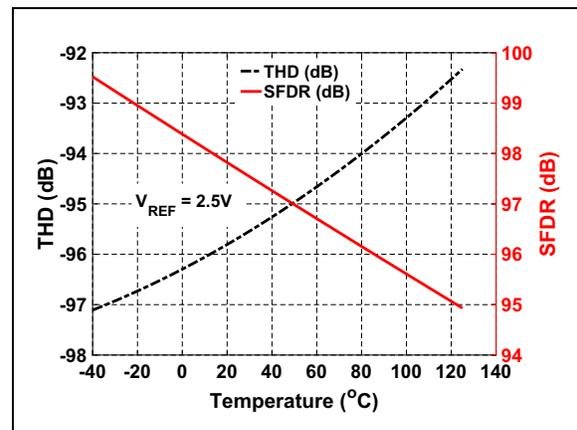
**FIGURE 2-23:** THD/SFDR vs. Temperature:  $V_{REF} = 2.5\text{V}$ .
