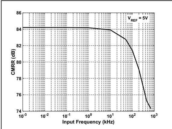
**FIGURE 3-31:** CMRR vs. Input Frequency:  $V_{REF} = 5\text{V}$ .
