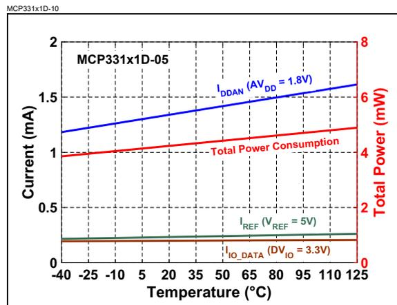
**FIGURE 4-36:** Power Consumption vs. Temperature:  $C_{LOAD\_SDO} = 20\text{ pF}$ .
