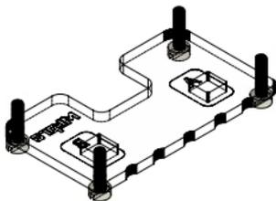
Push Large Screws through part number 1 and lay flat with text facing down.
