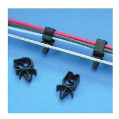
Integral "spring" holds wire bundles tightly. Used in pre-drilled .250" (6.4mm) diameter holes in panels up to .105" (2.7mm) thick. Vertical and horizontal versions available.
