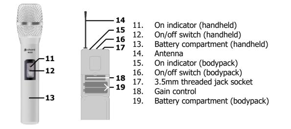
Note: If replacement transmitters are required, these must be genuine Chord branded transmitters which transmit the correct pilot tone to match with the receiver. Transmitters which have the same carrier frequency but not the correct pilot tone will not work with NU-20 receivers.
