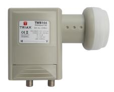
TWB 104 - Wideband LNB receives Ku satellite and generates a Horizontal and Vertical IF signal. Each output contains both the low and the high band of the polarization. The signal can be distributed to multiple STB's with wideband compatible tuners. The Wideband LNB can also be used in MDU's distributed by a dSCR MultiSwitch to multiple tuners that are not wideband compatible.
