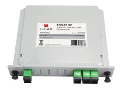
The optical splitter uses a planar light wave circuit (PLC) based on silica optical waveguide technology. It features small size, high reliability, wide operating wavelength range and good channel-to-channel uniformity. The splitter circuit is packaged in a plastic cassette and are terminated with SC/APC connectors. The cassette can be mounted:
