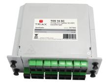
The optical splitter uses a planar light wave circuit (PLC) based on silica optical waveguide technology. It features small size, high reliability, wide operating wavelength range and good channel-to-channel uniformity. The splitter circuit is packaged in a plastic cassette and are terminated with SC/APC connectors. The cassette can be mounted:
