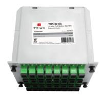
The optical splitter uses a planar light wave circuit (PLC) based on silica optical waveguide technology. It features small size, high reliability, wide operating wavelength range and good channel-to-channel uniformity. The splitter circuit is packaged in a plastic cassette and are terminated with SC/APC connectors. The cassette can be mounted in a 19" 3HU rack
