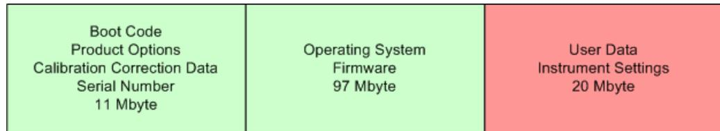
*Figure 4-1: Logical sections of the Flash memory*
