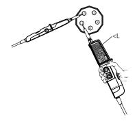
When re-testing with exchanged test probes theopposite symbol has to be illuminated.
