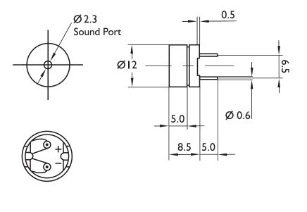
Requires additional electronic circuitry to operate as a sounder. Not wave solderable.
