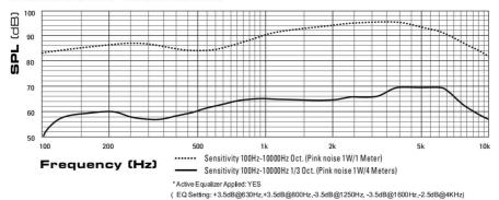
The SENTRY6RT/EN & SENTRY6RT/ENC have been tested for 100 hours at a maximum power of 6W. Both units did not deviate by more than +/- 3dB. The frequency response and impedance curves remained constant throughout the test period. All results are in full compliance with the requirements of EN54-24
