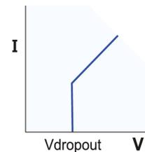
Resistive discharge (conductance mode) with voltage dropout.
