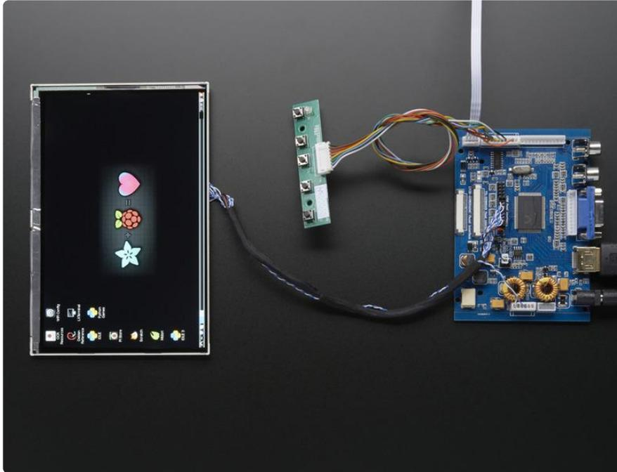
This is one of our prettiest display It's got excellent resolution (1280x800!) and IPS display so it is bright, crisp and looks good from any angle. This driver even has HDMI audio support and can drive two 4 ohm speakers directly.
