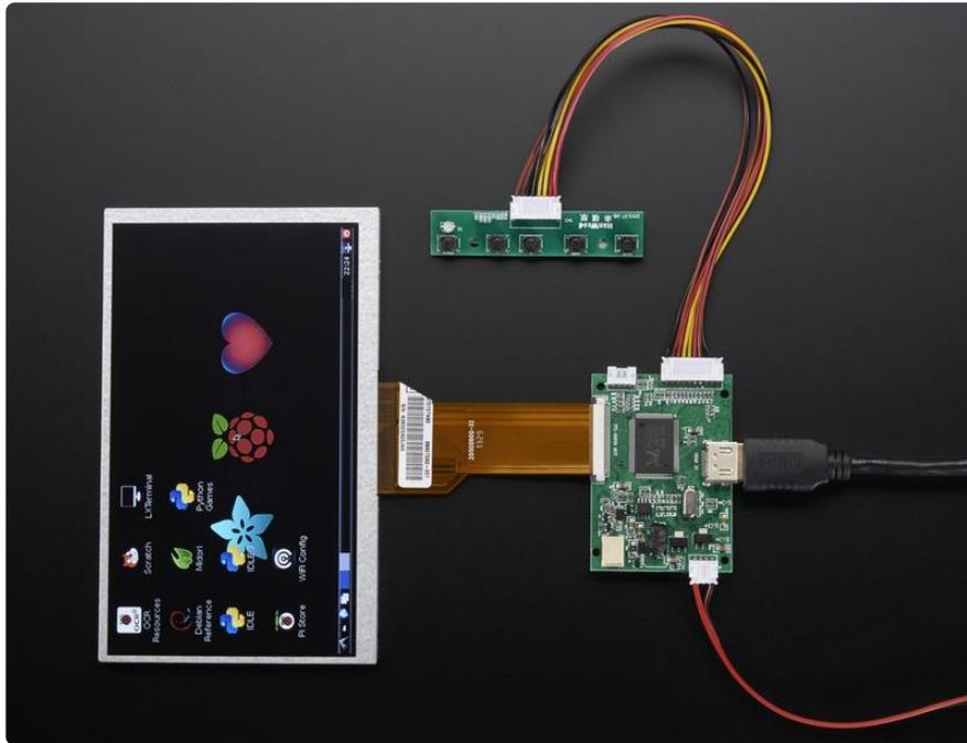
This is a medium sized, but easy to use HDMI-compatible displays, works great and is fairly small! The display looks nice and bright. We also have this display with a HDMI/VGA/NTSC/PAL driver (#1934)
