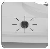
step the During temperature indicator light AUTOMATICALLY switches ON to show that the heating element is **OPERATIONAL** and heating up to the required temperature. Once the required temperature is reached the light will AUTOMATICALLY switch OFF indicating that it is READY for use.
