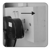
**2** CONNECT the mains cord to a suitable 220-240v~50/60Hz mains power supply.
