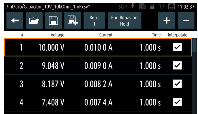
Arbitrary editor on the R&S®NGM200 power supplies.
