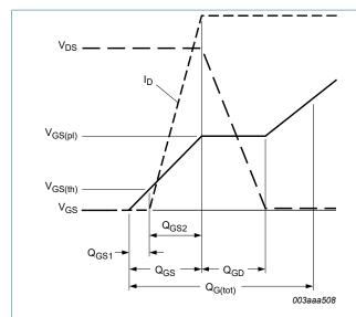
Fig. 13. Gate charge waveform definitions
