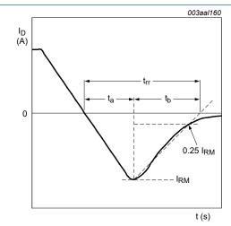
Fig. 16. Reverse recovery timing definition
