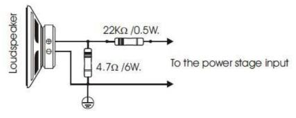
loudspeaker, install between the volume potentiometer and the loudspeaker following resistors according to the drawing hereafter.
