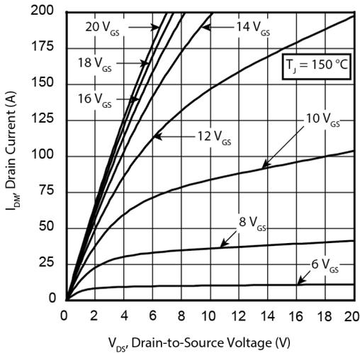
**Figure 4 • Drain Current vs. Drain-to-Source Voltage**
