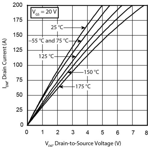
**Figure 2 • Drain Current vs. Drain-to-Source Voltage**
