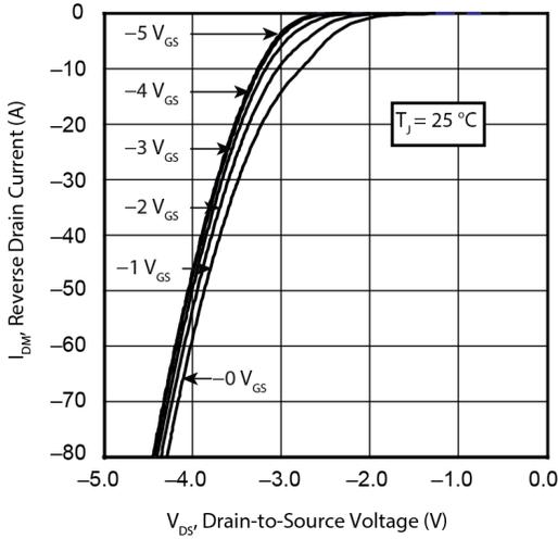
**Figure 10 • IDM vs. VDS Third Quadrant Conduction**
