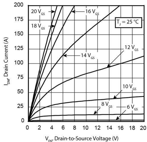
**Figure 3 • Drain Current vs. Drain-to-Source Voltage**
