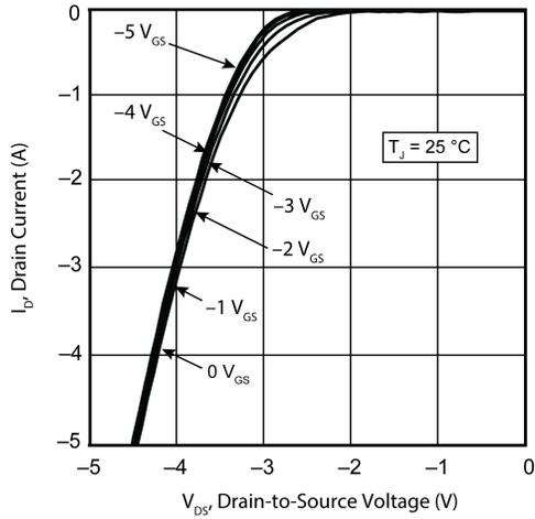
Figure 9 •  $I_D$  vs.  $V_{DS}$  3<sup>rd</sup> Quadrant Conduction
