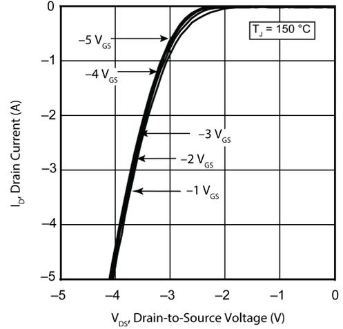
Figure 10 •  $I_D$  vs.  $V_{DS}$  3<sup>rd</sup> Quadrant Conduction
