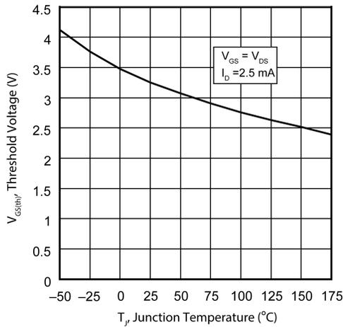
Figure 15 • Threshold Voltage vs. Junction Temp.
