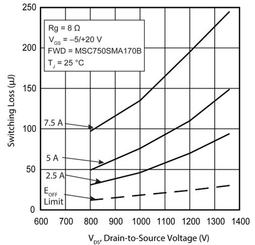
Figure 12 • Switching Energy vs.  $V_{DS}$  &  $I_D$
