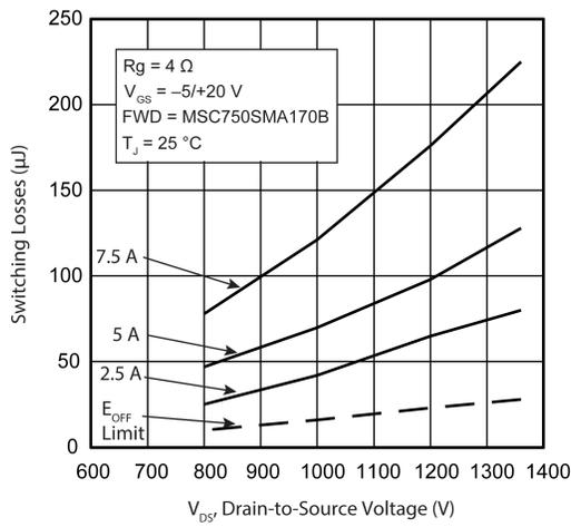
Figure 11 • Switching Energy vs.  $V_{DS}$  &  $I_D$
