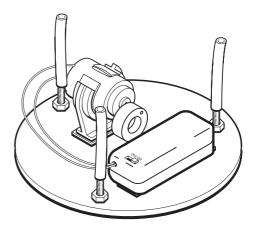
9. Turn ON the switch and stand your Bug on a firm surface. It should move around as it vibrates.
