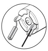
8. Attach the clear plastic legs to the bug by pressing and twisting them onto the screws.
