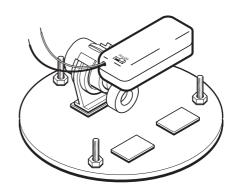
7. Connect the battery wires to the motor using the sleeves as shown. Just push the wires through the tags. DO NOT TRY TO TWIST THEM.
