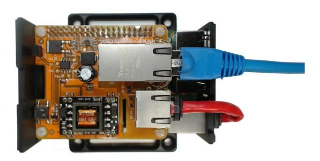
**Step** 8 – Slide the top part of the case back in place. As you do that gently pull out each side of the top part of the case so to allow the connectors of the Raspberry Pi to slot into place.
