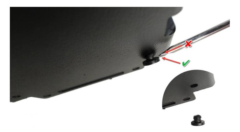
**Step 4** – Currently the case will fit together with a Raspberry Pi 4 but there are also some cutouts that can be pushed through to allow compatibility with the 3B+ and models below this. Take a small pointed tool such as a screwdriver and push through cutout. This will allow the HDMI connector to become accessible.
