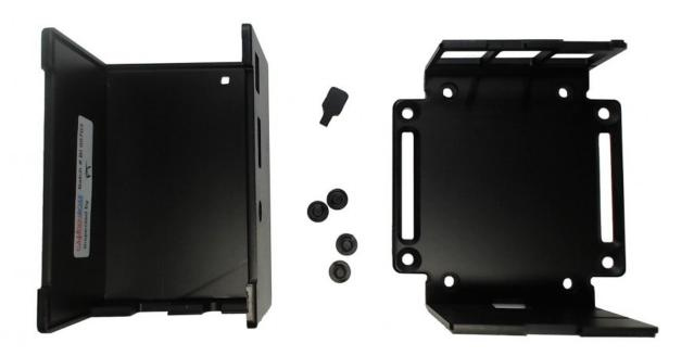
Step 2 – Insert the plastic button extender through the hole of the top part of the case.
