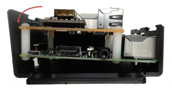
The PCBs of the two boards should be aligned within the grooves of the panel as shown in the picture.
