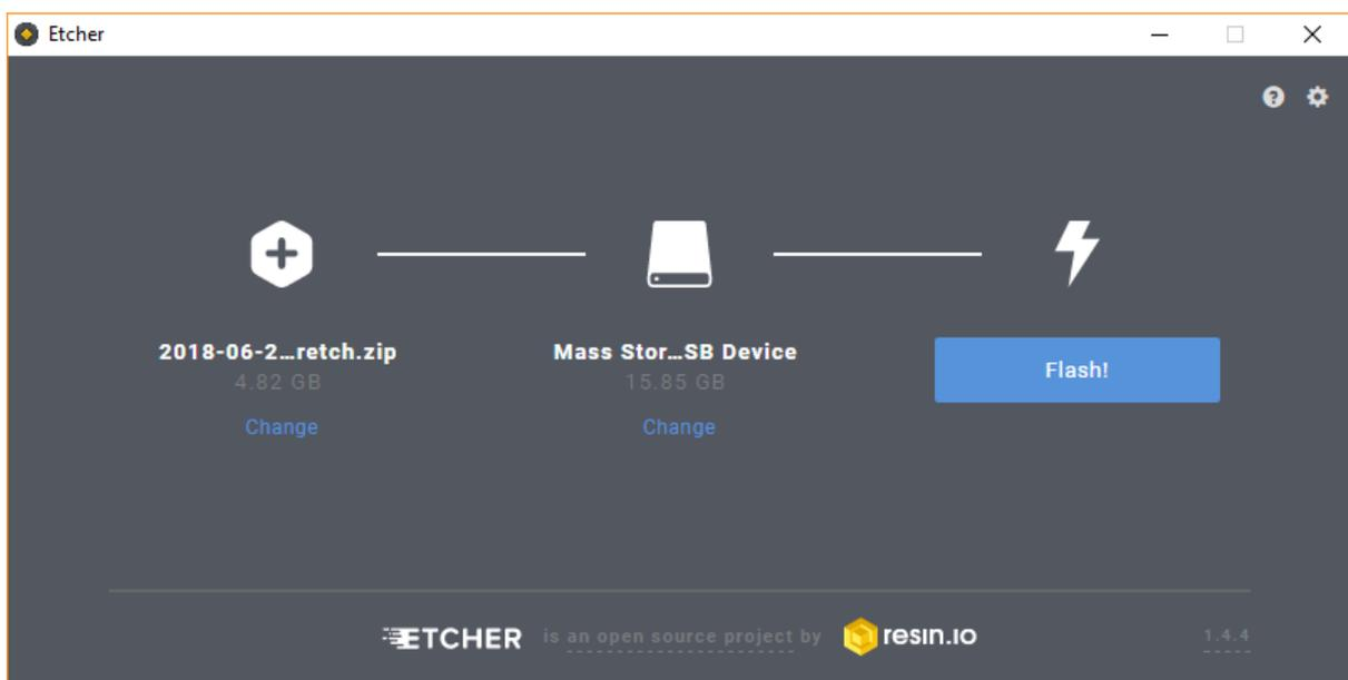
After done flashing, take the [SD card](#) out and insert back to your laptop. Open [SD card](#) directory (e.g. D:/boot) and open **config.txt** file. Put **enable\_uart=1** at the bottom of the line. Save and eject the [SD card](#). Then insert the [SD card](#) into [Raspberry Pi Zero WH](#).
