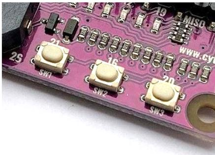
3 units of programmable push button are included in the Maker pHAT. To utilize it, user need to configure push button GPIO as input pullup.
