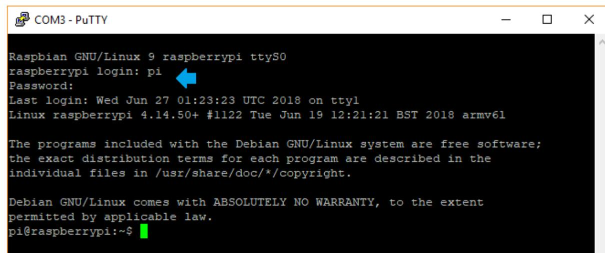
So far, you're able to access Raspberry Pi through serial remote (Maker pHAT). We will further guide you until we can remote using [VNC Viewer](#) (Virtual Network Computing).
