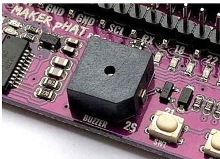
Maker pHAT also comes with on-board active buzzer. It is standard output digital device connected to GPIO 26. To activate it, set GPIO to high, and to mute it, just set GPIO to low.
