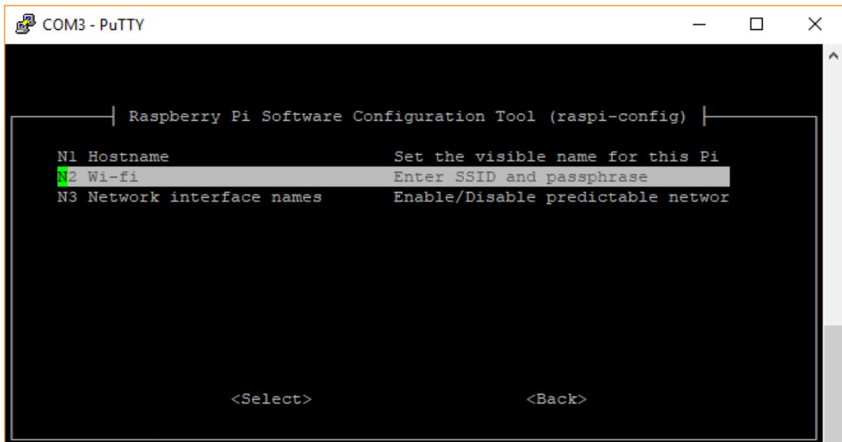
The screenshot shows the 'Raspberry Pi Software Configuration Tool (raspi-config)' Network Options menu. The menu lists three options, with 'N2 Wi-fi' highlighted. The options are:
