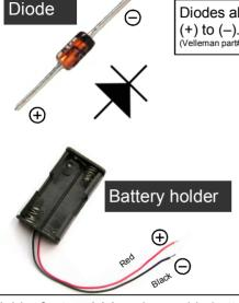
Diodes allow the current to flow in only one direction, from (+) to (–). Current flow in the opposite direction is blocked. (Velleman part# BAT85)
