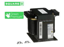
Transformer, Type T, industrial control, 750 VA, 240/480 VAC primary / 120/240 VAC sec, 1 phase, 50/60 Hz, 115 °C rise
