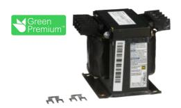
Transformer, Type T, industrial control, 350 VA, 240/480 VAC primary / 120 VAC secondary, 1 phase, 50/60 Hz, 80 °C rise
