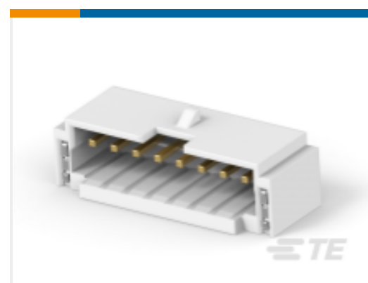
TE Part # 2-2381626-8 1.5P 8POS WTB R/A BRD W LATCH AU NAT
