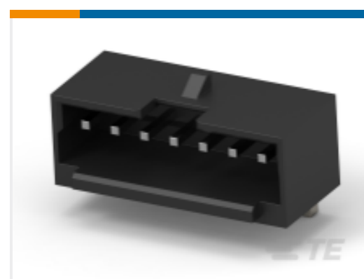
TE Part # 4-2380320-7 1.5P 7POS WTB VERT BRD W LATCH TIN BLACK
