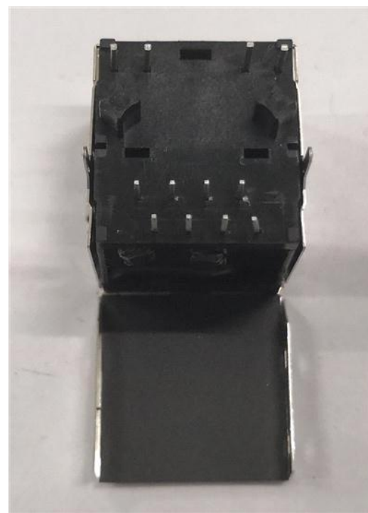
Above: Using a plastic plate instead of a thin tape to separate cores from Shielding.
