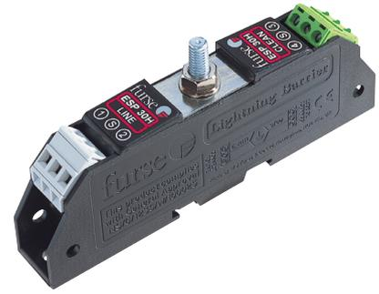
Combined Category D, C, B tested protector (to BS EN 61643) suitable for most twisted pair signalling applications. Available for working voltages of up to 6, 15, 30, 50 and 110 Volts. ESP TN suitable for Broadband, POTS, dial-up, T1/E1, lease line and \*DSL telephone applications. For use at boundaries up to LPZ 0 to protect against flashover (typically the service entrance location) through to LPZ 3 to protect sensitive electronic equipment.
