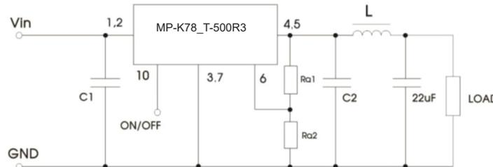
Fig. 3 External "LC" output filter circuit diagram
