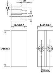
Tightening torque 15Nm max.
