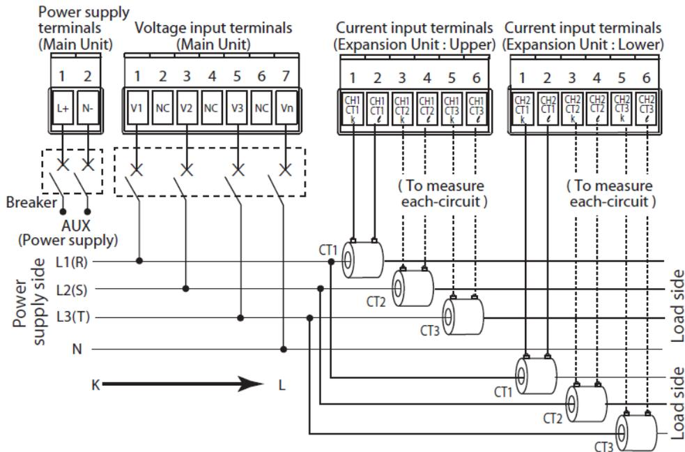
**!** Vn terminal should be connected to N-phase which is grounded.
