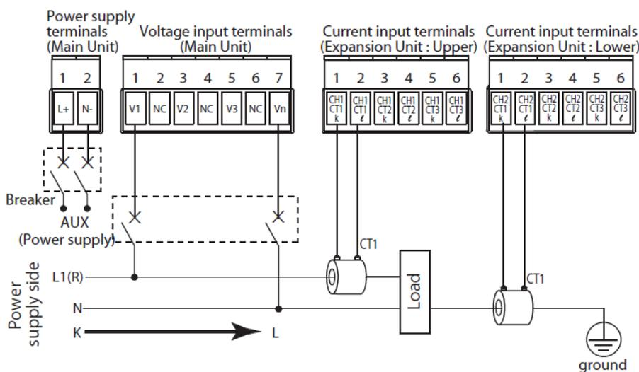
By inputting the ground line of the equipment to CT input or direct current input, it is possible to measure the leakage current of the ground, and it can be used as equipment maintenance.
