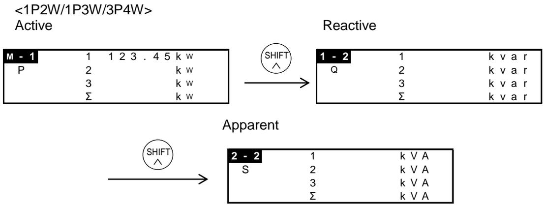
•Eco-POWER METER displays the power as below.
