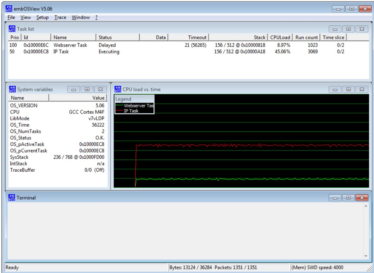
Most often, a serial interface (UART) is used for the communication with the target hardware. Alternative communication channels include Ethernet, memory read/write for Cortex-M and RX CPUs, as well as DCC for ARM7/9 and Cortex-A/R CPUs. The hardware dependent routines and defines available for communication with embOSView are implemented in the source file `RTOSInit.c`. Details on how to modify this file are also given in chapter *Setup target for communication* on page 425.
