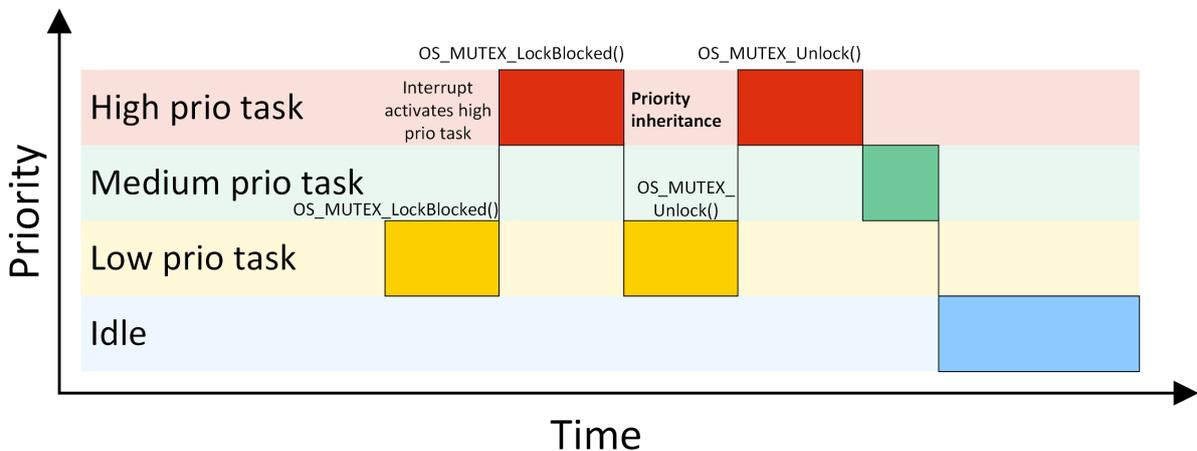
With priority inheritance, the low priority task inherits the priority of the waiting high priority task as long as it holds the mutex. The lower priority task is activated instead of the medium priority task when the high priority task tries to claim the semaphore.
