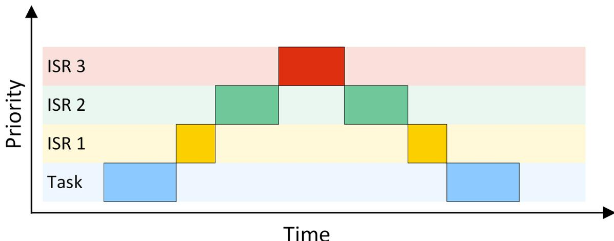
For applications requiring short interrupt latency, you may re-enable interrupts inside an ISR by using `OS_INT_EnterNestable()` and `OS_INT_LeaveNestable()` within the interrupt handler.
