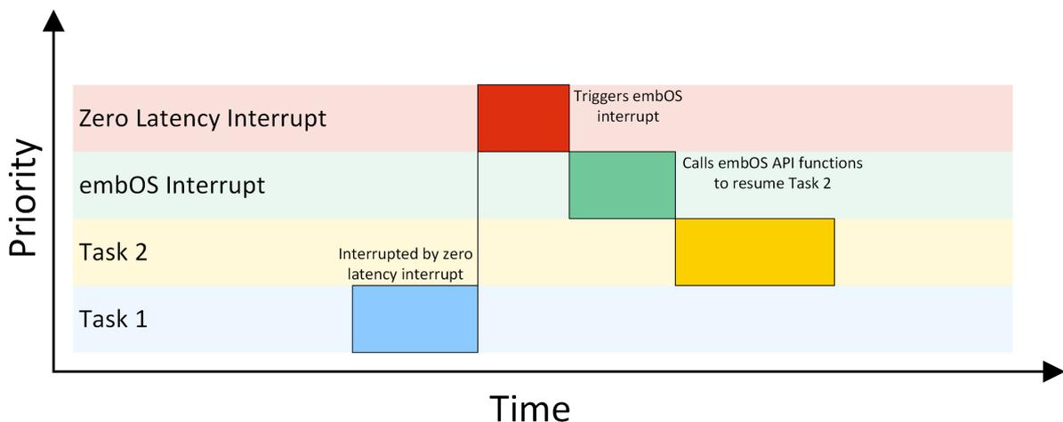
The task 1 is interrupted by a high priority interrupt. This zero latency interrupt is not allowed to call an embOS API function directly. Therefore the zero latency interrupt triggers an embOS interrupt, which is allowed to call embOS API functions. The embOS interrupt calls an embOS API function to resume task 2.
