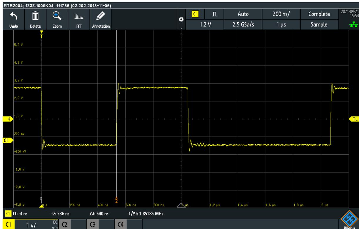
$t_{AB}$  is measured as 540ns.
