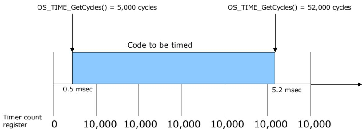
The first call to `OS_TIME_Get_Cycles()` returns the starting value at 5,000 cycles, while the second call to `OS_TIME_Get_Cycles()` returns the ending value at 52,000 cycles. The measured execution time of the code in this example would therefore be  $(52,000 \text{ cycles} - 5,000 \text{ cycles}) = 47,000 \text{ cycles}$ , which exactly equals 4.7 millisecond.
