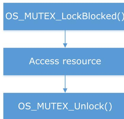
A mutex contains a counter that keeps track of how many times the mutex has been claimed by calling `OS_MUTEX_Lock()` or `OS_MUTEX_LockBlocked()` by a particular task. It is released when that counter reaches zero, which means the `OS_MUTEX_Unlock()` routine must be called exactly the same number of times as `OS_MUTEX_LockBlocked()` or `OS_MUTEX_Lock()`. If it is not, the mutex remains blocked for other tasks.
