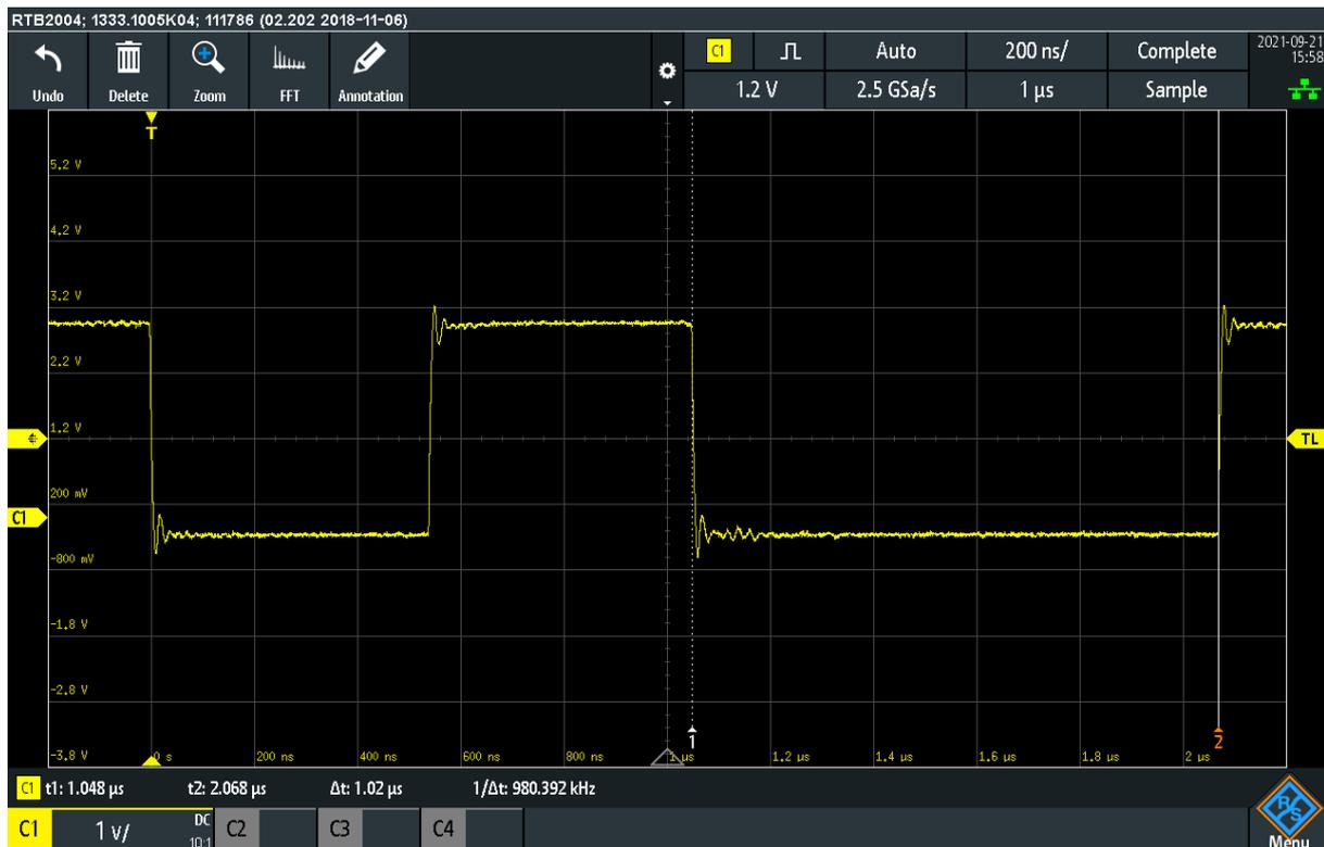
$t_{CD}$  is measured as 1020ns.
