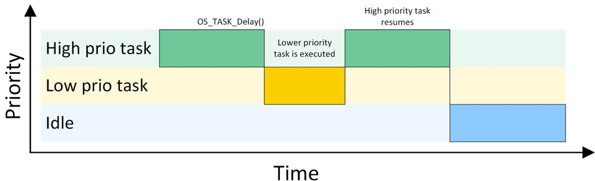
If tasks in a pure cooperative multi-tasking system do not cooperate, the system “hangs”. This means that other tasks have no chance of being executed by the CPU while the first task is being carried out. Even if an ISR makes a higher-priority task ready to run, the interrupted task will be resumed and completes before the task switch is made.
