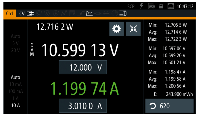
DVM display on an R&S ® NGM200 power supply.
