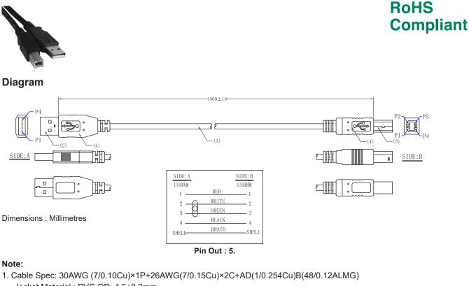
1. Cable Spec: 30AWG (7/0.10Cu)×1P+26AWG(7/0.15Cu)×2C+AD(1/0.254Cu)B(48/0.12ALMG) Jacket Material : PVC OD: 4.5±0.2mm Colour : Black
