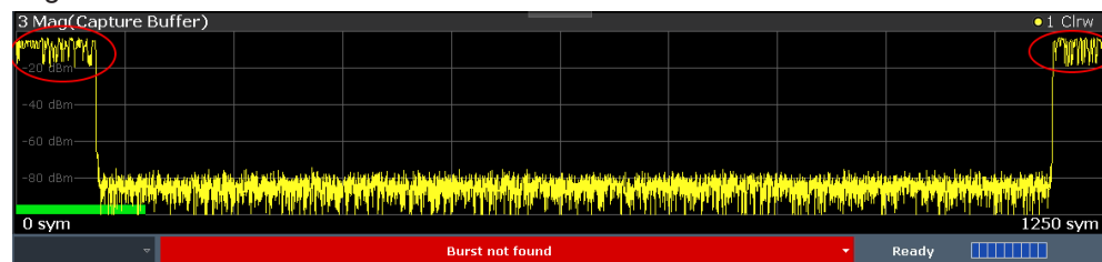
Figure 10-2: Example for incomplete burst capture
