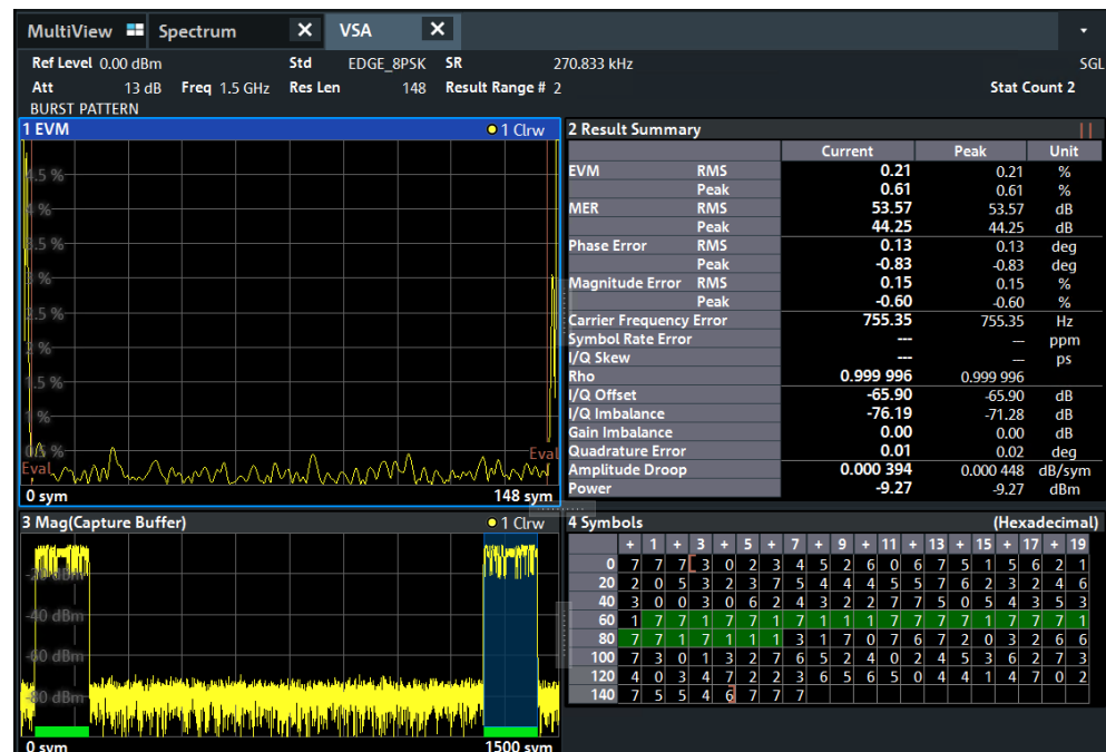
Figure 9-6: Default display configuration for GSM 8PSK EDGE
