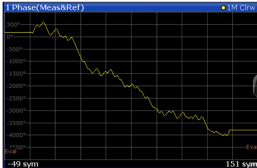
Figure 3-20: Phase Unwrap result display
