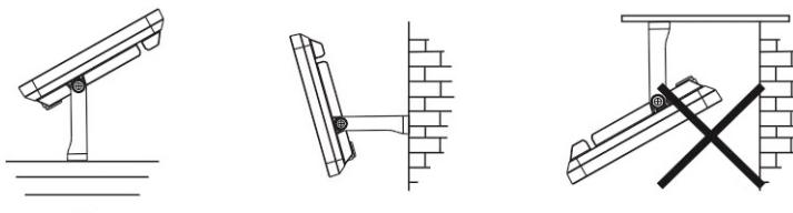
The floodlight has a beam angle of 120°. It can be tilted upwards and downwards at an angle of approximately 90°. The angle of adjustment will vary slightly between models.
