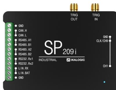
Figure 2: sp209i logic analyzer (industrial version)
