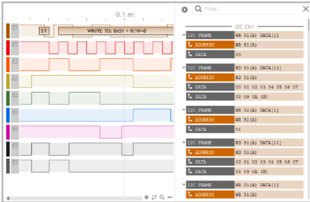
Figure 3: Example of logic signals captured and analyzed by SP209 logic analyzer
