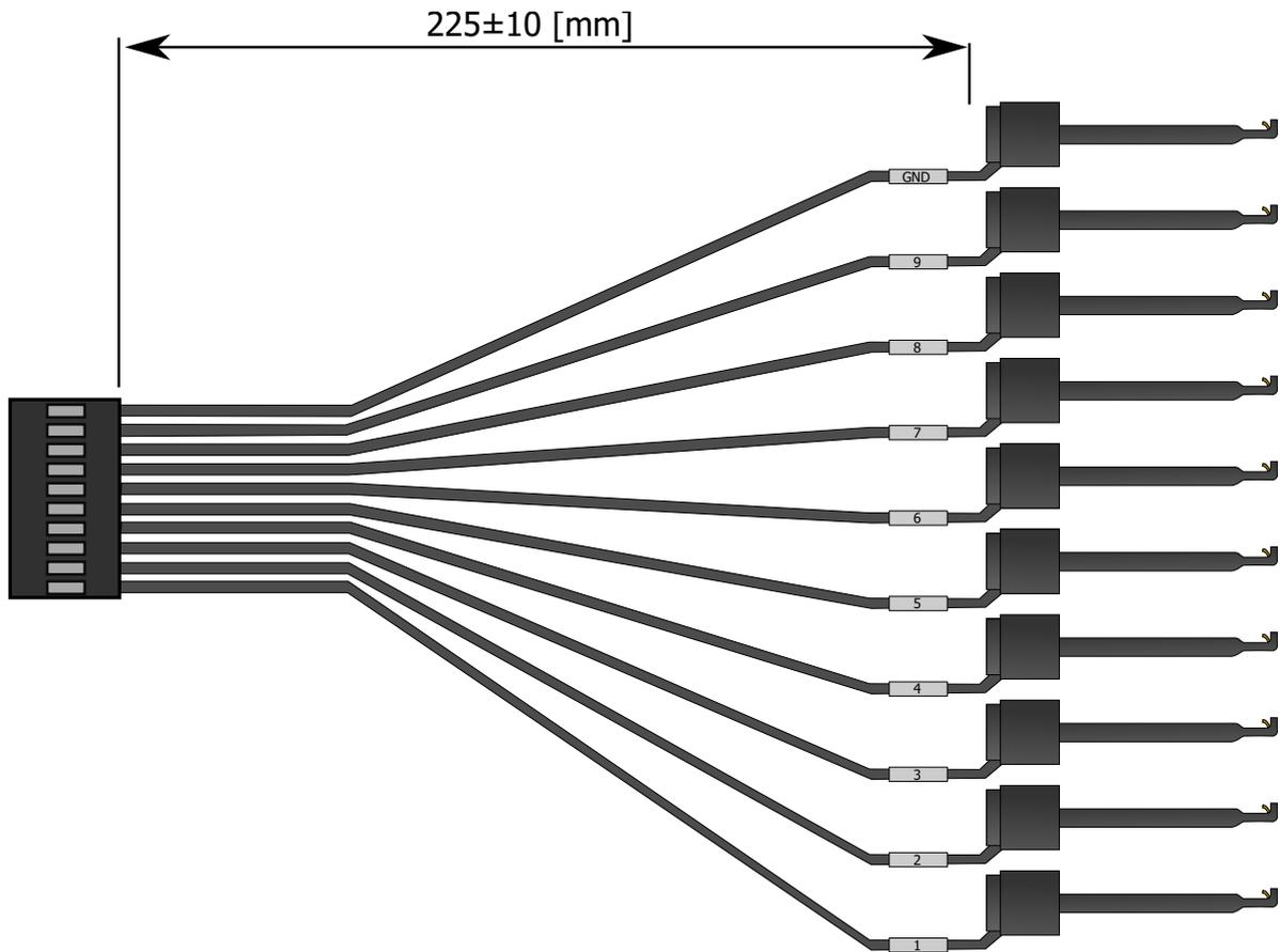
Figure 9: Probes dimensions (mm)
