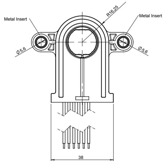
Sensor shown above is the 17mm version with the rotor at zero position. Sensor is delivered at random position. Wires: 0.35mm<sup>2</sup> TXL SAE J1128
