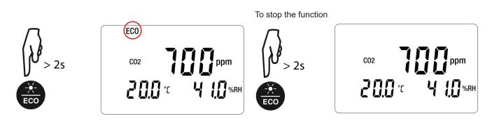
In the ECO mode, the measurement is more sensitive to instantaneous variations of  $CO_2$ . For example, if the user breathes near the device, it may throw off the measurement. It will be necessary to wait for the next measurement to recover the true concentration of  $CO_2$  in the room.
