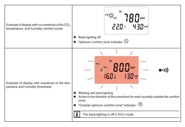
For the **1D** and **3D** modes, if the buzzer is active, it will sound intermittently upon the appearance of the O symbol.
