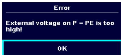
In pre-test a too high external voltage was detected between P and PE terminals. The measurement was cancelled. Press **OK** to continue.
