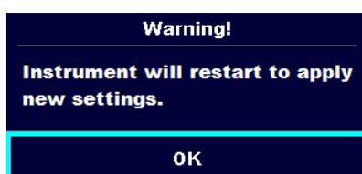
Warning for restart of the instrument to set new Ethernet settings. This message appears on exit from Settings menu after changing Ethernet settings. Press **OK** to continue.
