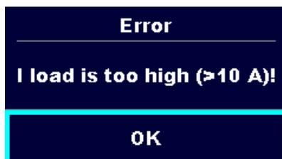
The load current exceeded the highest upper limit of 10 A for the Discharging time test. Measurement was aborted. Press **OK** to continue.
