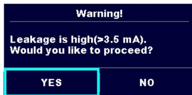
In pre-test a possible high leakage current was detected. It is likely that a dangerous leakage current (higher than 3.5 mA) will flow after applying power to the device under test.
