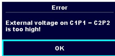
In pre-test an external voltage between C1/P1 and C2/P2 terminals was detected. The measurement was cancelled. Press **OK** to continue.
