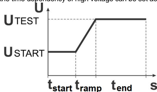
Figure 6.28: Voltage / time diagram of the HV AC programmable test
