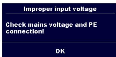
Warning for improper supply voltage condition. If pressing **OK** instrument will continue to work in a limited mode (measurements are disabled).
