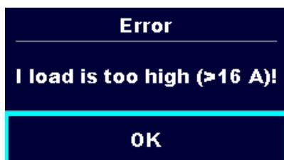
The load current exceeded the highest upper limit of 16 A for the Power and Leakage tests. Measurement was aborted. Press **OK** to continue.
