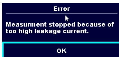
The measured leakage ( $I_{diff}$ ,  $I_{pe}$ ,  $I_{touch}$ ) current was higher than 20 mA. Measurement was aborted. Press **OK** to continue.
