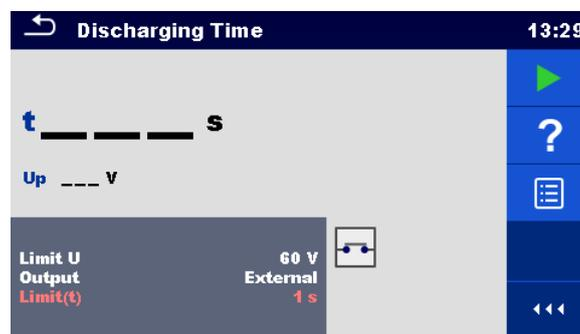
Figure 6.60: Discharging Time test menu
