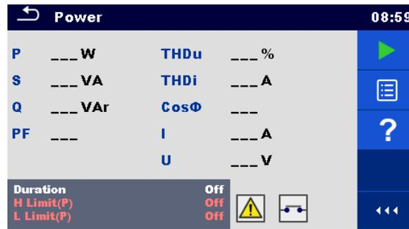
Figure 6.54: Power measurement menu
