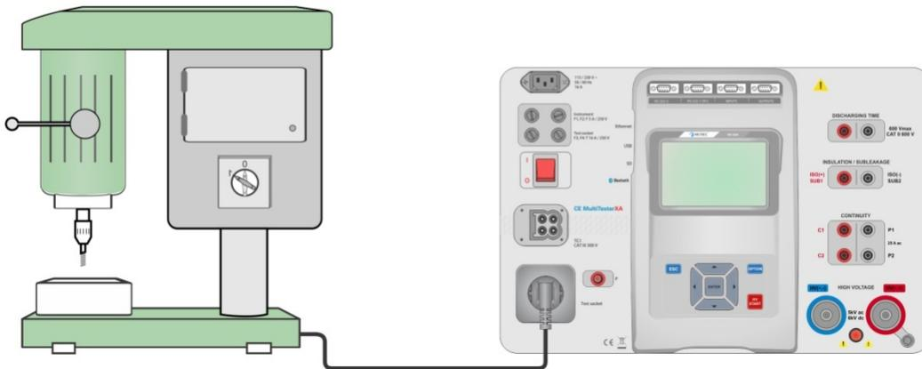
Figure 6.64: Discharging Time test (Output = Socket)
