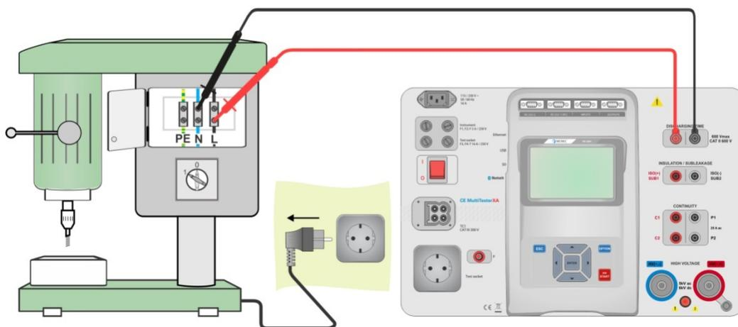
**Figure 6.62: Discharging Time test (Output = External)**
