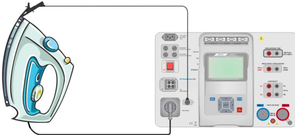
Figure 6.18: Measurement of Continuity P/S - PE
