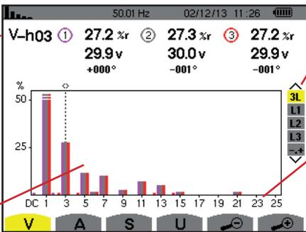
Display of the 3 phases 3L, of L1, L2, L3, N, or (for the C.A 8333 only) of the expert mode (three-phase connection only - see §6.5). To select the display press the ▲ or ▼ key.
