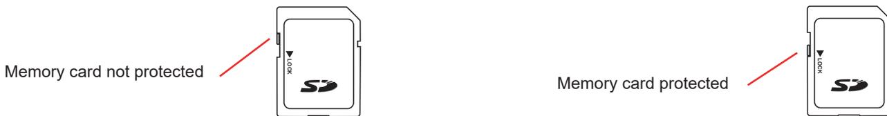
To withdraw the memory card from its space, proceed as for the replacement of the battery, described in §17.3. Once the battery has been withdrawn from its compartment, push the tab out of the way, then push the memory card out of the device. To put the card back in place, slide it horizontally into its space until it is home and the tab is back in position.
