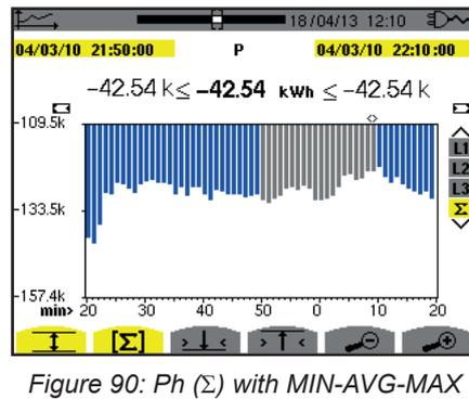
With the MIN-AVG-MAX mode activated, the display differs slightly from the previous one because there is no loss of information.
