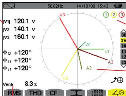
Discs indicating potential saturation of the channel.
