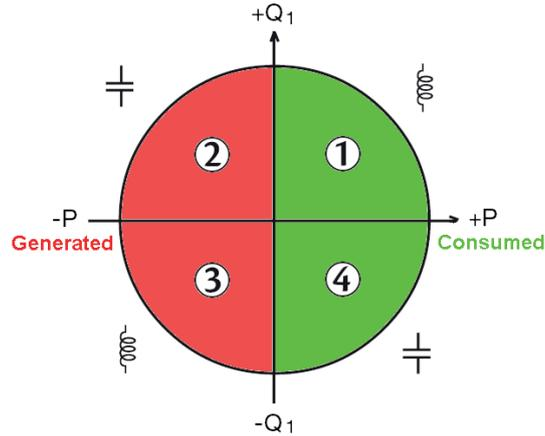
Figure 111: Four-quadrant diagram
