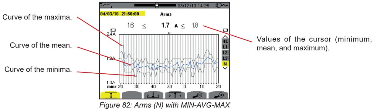
The display period of this curve is one minute. Each point of the mean curve represents the arithmetic mean of 60 values recorded every second. Each point of the curve of the maxima represents the maximum of the 60 values recorded every second. Each point of the curve of the minima corresponds to the minimum of the 60 values recorded every second.
