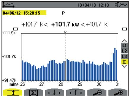
Figure 88: P ( $\Sigma$ ) with MIN-AVG-MAX
