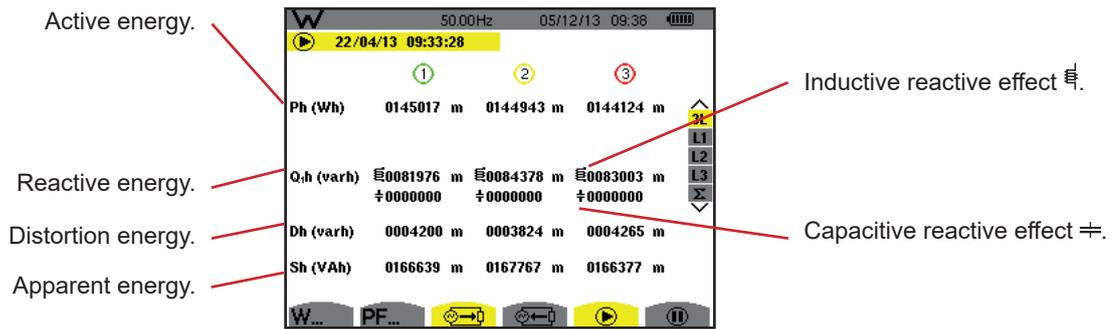
Figure 99: The Energies Consumed display screen in 3L
