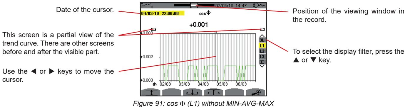
The period of display of this curve is two hours. Since the recording period is one second, each point of this curve represents a value recorded every second taken every two hours. There is therefore a substantial loss of information (7,199 out of 7,200), but the display is rapid.
