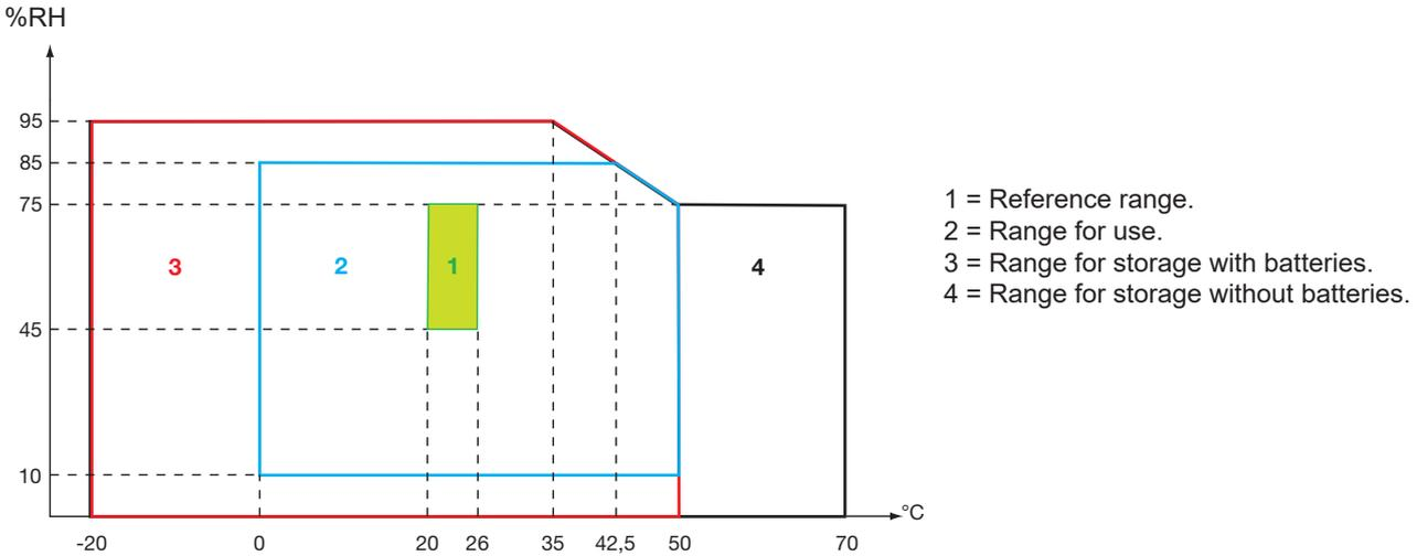
**Caution:** at temperatures above 40°C, the device must be powered by the battery alone **OR** by the mains power unit alone; use of the device with both the battery **AND** the mains power unit is **prohibited**.
