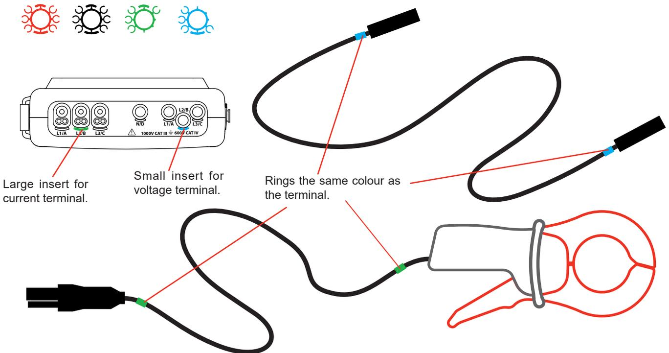
Figure 10: Identification of the leads and terminals
