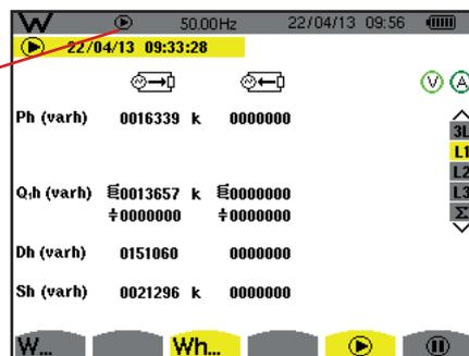
Figure 106: The Energy Metering screen in varh
