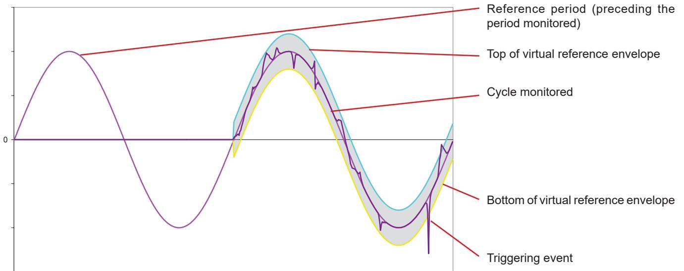
The half-width of the virtual envelope for the voltage and current is equal to the threshold programmed in the Transient mode of the configuration (see §4.8).
