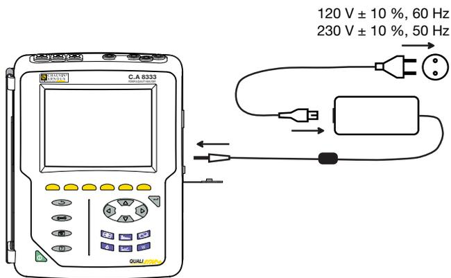
Remove the cover from the receptacle and connect the plug of the specific power supply unit to the device. Connect the mains cord to the power supply unit and to mains.
