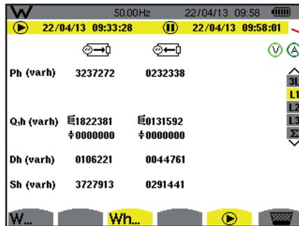
The stop date and time of the metering are displayed alongside the start date and time.
