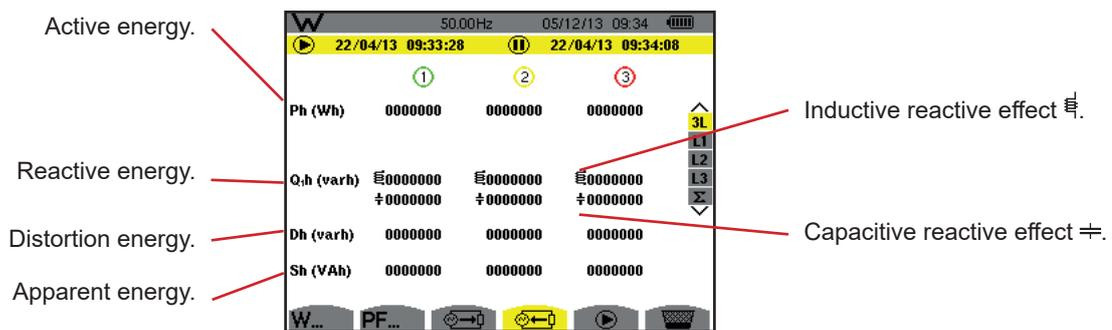
Figure 100: The Energies Generated display screen in 3L
