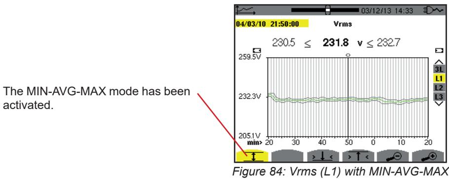
This curve differs slightly from the previous one because, with the MIN-AVG-MAX mode, there is no loss of information.
