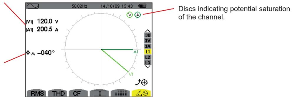
Figure 72: The L1 Fresnel diagram display screen
