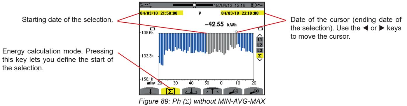
The display period of this bar chart is one minute. Since the recording period is one second, each bar of this bar chart represents a value recorded in a one-second window once a minute.
