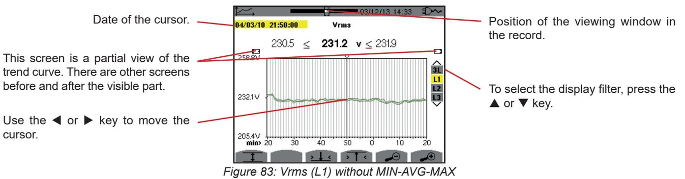
For each of the phases (L1, L2, and L3), at each recording of a value over one second (recording period), the device also records the minimum half-cycle RMS value over one second and the maximum half-cycle RMS value over one second. These are the three curves shown in the figure above.
