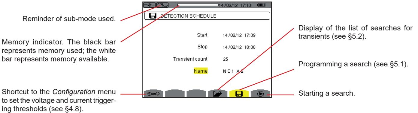
Figure 37: The *Detection schedule* screen in Transient mode
