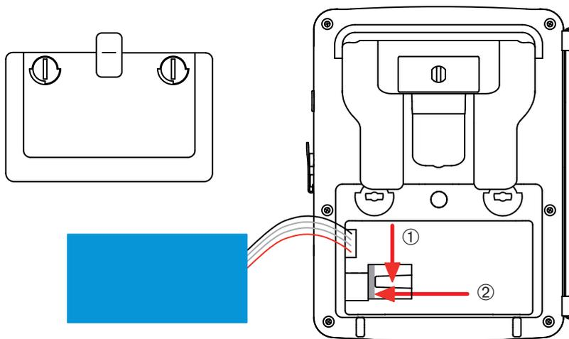
Then replace the battery and the battery compartment cover as explained in §17.3.
