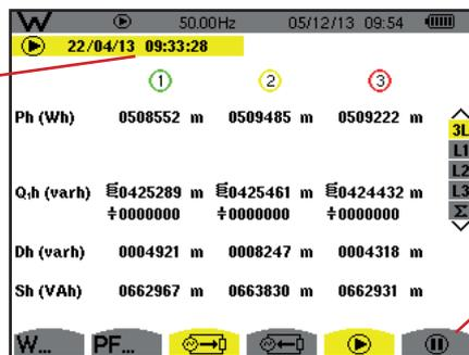
Figure 105: The Energy Metering Start-up screen in Wh
