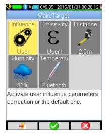
When user compensation is selected, the various parameters can be adjusted:
