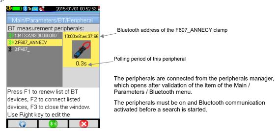
This manager lists the peripherals previously or currently connected. The peripherals connected are preceded by the icon while the peripherals that are not connected are preceded by .
