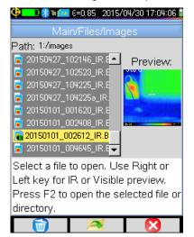
The file manager lists only infrared images generated by the camera bearing a name in the form vvvvmmdd hhmmssX IR BMP along with the folders to
