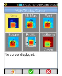
By default, no measurement cursor is selected (selection of the item in the Main/Display/Cursor menu), and the camera produces only infrared images.
