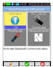
To use this function, you must first activate it from the Main/Parameters/Bluetooth menu by setting the Activation
