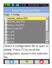
A setup file is recalled from the Main/Setup/User/Files menu, by means of the file manager, which lists all of the configuration files (extension .CFG) found in directory 1:/config/.
