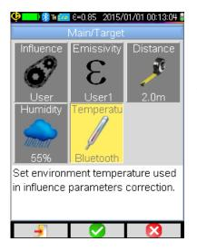
The measurements replace the user data entered in the Main/Target menu, provided that user influence is selected (see § 3.2.2. <u>Using the user compensation for the influencing factors</u>).
