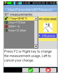
For the measurement to be used as an **influence**, the use "influence" must be assigned to it in the Bluetooth measurements viewing window
