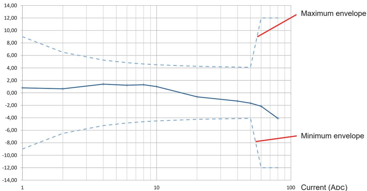
Typical amplitude error curve for a 60Hz AC current, 10mV/A range
