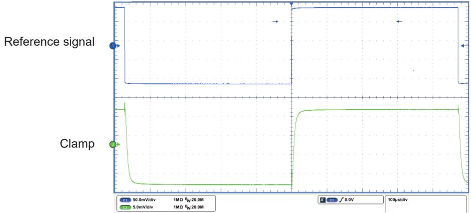
Pulse response at  $\pm 0.5 A_{peak}$  at the frequency of 1 kHz in the 1V/A range
