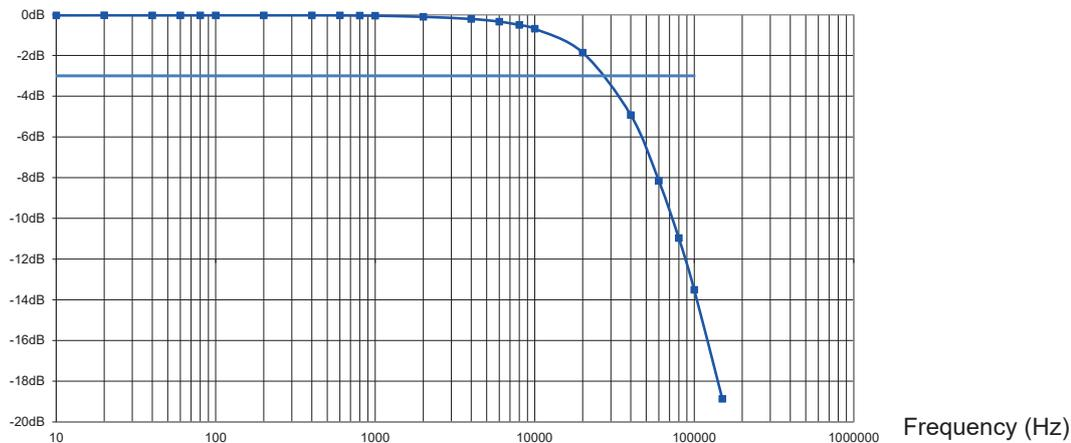
Typical amplitude error curve as a function of frequency,  $I = 0,5A$ ,  $1V/A$  range
