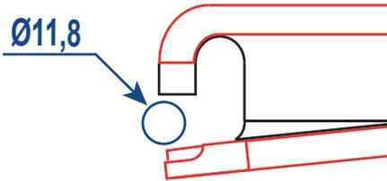
Clamping capacity: 11.8mm in diameter
