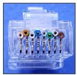
Smaller diameter in-line conductor design
