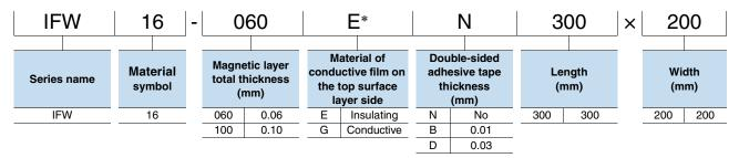
\* Note: If you don't need double-sided adhesive tape, there is no specification difference between E and G. (IFW16-060EN is equal to IFW16-060GN)
