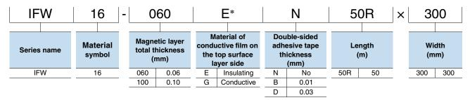
\* If you don't need double-sided adhesive tape, there is no specification difference between E and G. (IFW16-060EN is equal to IFW16-060GN)
