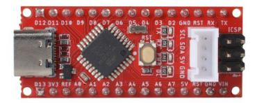
The Seeeduino Nano is a compact board similar to the Seeeduino V4.2/Arduino UNO, and it is fully compatible with Arduino Nano on pinout and sizes.
